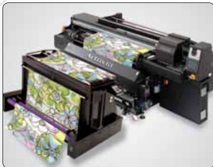
ST-4100 can be used as in-line unit or as stand-alone printer.
